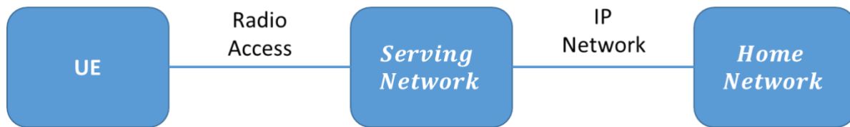
Figure 3 - Cellular Network Architecture
