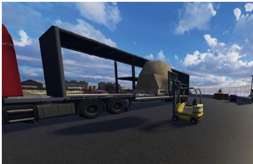
Figure 5: AGV after unloading of the truck waiting for the trajectory to follow
